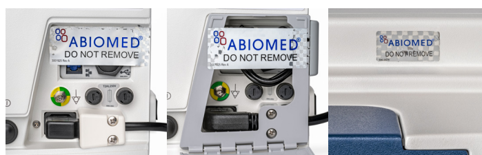
Figure 5.6 Automated Impella Controllers with evidence of tampering
