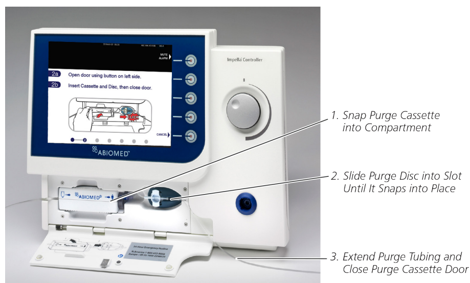
Figure 5.8 Inserting the Purge Cassette into the Automated Impella Controller
