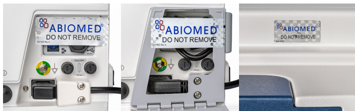
Figure 5.6 Automated Impella Controllers with evidence of tampering
